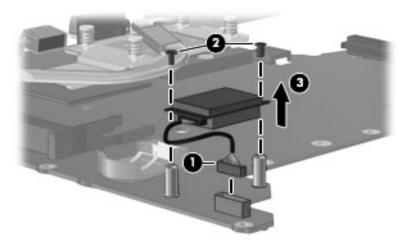
Reverse this procedure to install the Bluetooth module.
